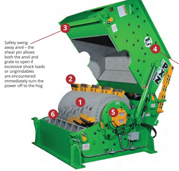
Hog case is fabricated using 1½" steel plate. All internal wear surfaces are covered with easy to replace bolt on internal case liners with clam shell opening to allow for safe and easy maintenance access.
