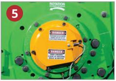
The bearing housing assembly is designed to be maintenance friendly allowing for simple removal and installation of hog bearings.
