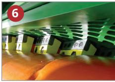
Heavy duty reinforced grate assembly with rotatable grate liner. Optional grate patterns are available for different applications and end product requirements.
