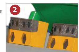
Bolt-on rotatable, Rocwear striker system. The patented Rocwear strikers provide the customer with two cutting edges per bit. Once one side is worn, the bit needs to be simply rotated thus doubling the life of each bit.
